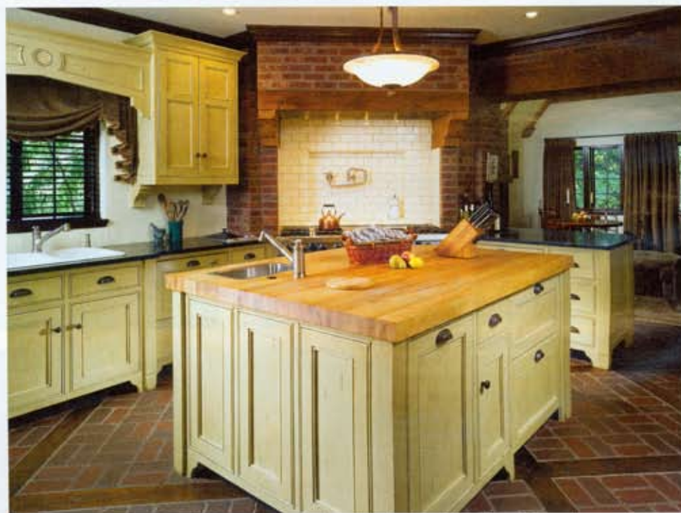
A maple countertop was placed in front of an oven and range to obscure a direct view of the modern appliance upon entry to the kitchen; the stainless-steel hood liner above is concealed with brick and French oak.
